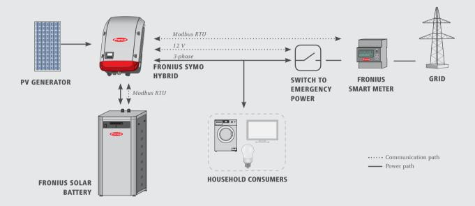
/ The Fronius Smart Meter is compatible with all inverters with an RS485 interface (Modbus RTU). The Fronius Smart Meter works in conjunction with the Fronius Datamanager 2.0 for the Fronius IG Plus inverters. The Fronius Smart Meter can be retrofitted at any time together with the Fronius Datamanager 2.0 in inverters that have already been installed.
